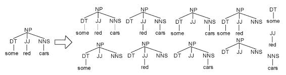
Fig. 2. Syntactic parse tree and all of its 11 subtrees covered by the convolution tree kernel.
